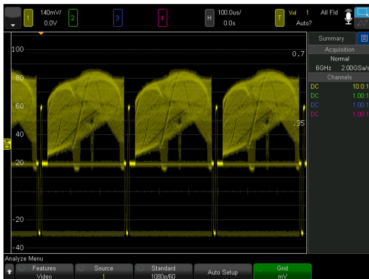
Figure 45. Triggering on a 1080p/60 signal.
