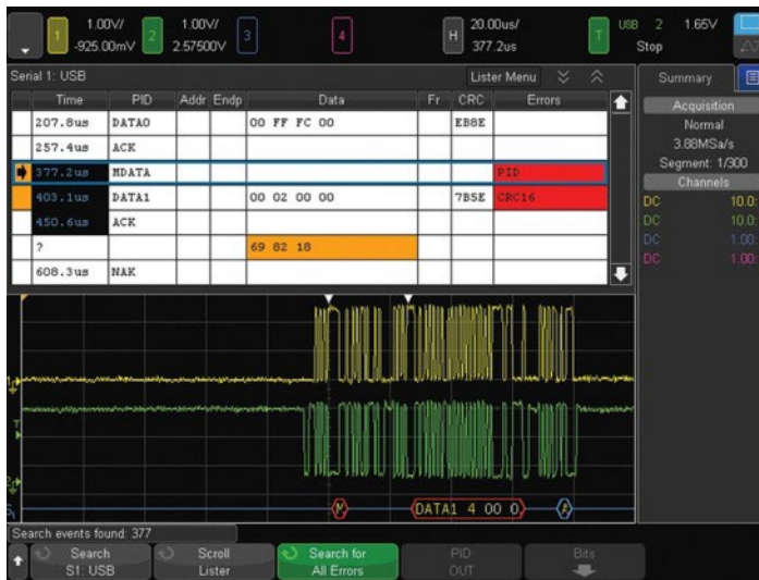
Figure 21. USB 2.0 trigger, decode and "lister" display.
