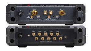
Only the 4-port ECal modules (i.e. N4431/32/33D) are supported for multiport calibration with the S97553B.
