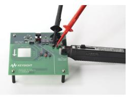
The Keysight U1880A deskew fixture allows you to quickly deskew your voltage and current probes, enabling accurate and precise power measurements.
