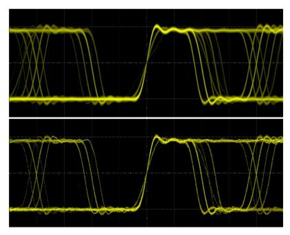
This is a comparison of the EXR-Series (top) vs. another oscilloscope, each viewing the same signal with identical settings. The lower photo is an oscilloscope triggering under 1,000 wfm/s, with one second of persistence enabled. How many signal details would you miss if you were using the oscilloscope on the bottom instead of the EXR-Series?
