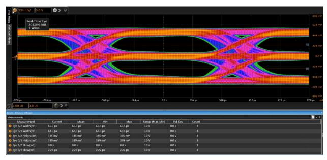
This package quickly sets up clock recovery and measurements for a PAM-encoded signal. The software can accurately set the individual threshold levels of your PAM signal and render each individual eye. It also includes BER/SER measurements and statistics.
