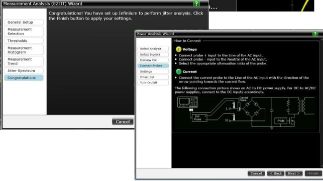
For more complex tests, there are Setup Wizards. These step-driven dialog boxes walk you through fine-tuning your analysis even further, explaining different features and settings in more detail. Setup Wizards are available for power analysis, power integrity, real-time eye diagrams, jitter decomposition, measurement analysis (trends, histograms, etc.), crosstalk, and more!
