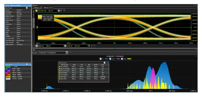
This package offers advanced statistical analysis of high-speed digital interfaces in the vertical (voltage) and horizontal (time) domains, as well as phase noise analysis. The result: the industry's most complete jitter and noise analysis software for real-time oscilloscopes.
