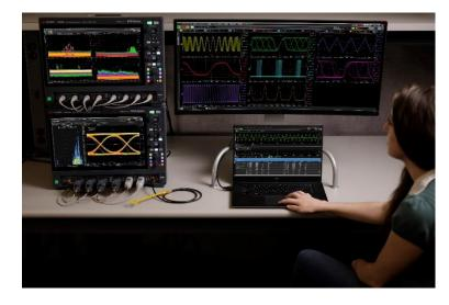
MultiScope is a standard feature of the EXR-Series oscilloscope and of Infiniium Offline – the only requirement to combine two oscilloscopes is the cabling kit. Specifications for frame-to-frame jitter, setup instructions, and ordering information can be found in the MultiScope Brochure and User's Guide. Simply search for "MultiScope" on our website or look in the technical documentation on your oscilloscope model's product page.
