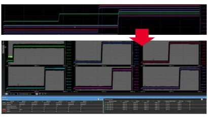
With waveforms separated into grids and independent mask tests possible on every channel, you can continuously test six power rails over thousands of startup cycles. Notice how there are mask tests and measurement results on screen for a single screen shot test report.
