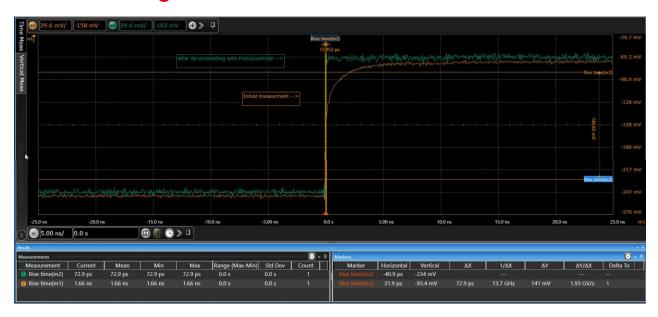
This package includes PrecisionProbe and InfiniiSim Basic, two tools designed to de-embed the effect of cables and fixtures from measurements. PrecisionProbe characterizes the response of a probe, cable, or fixture. InfiniiSim enables you to model them out of a measurement.
