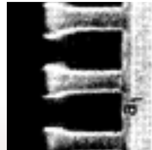
Ammonia and amines can interact with acid catalyzed photoresists, resulting in t-topping
