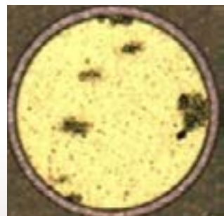
Acidic gases can cause corrosion of precision metallic thin films
