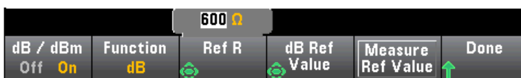
Figure 6. Automatic scaling provides a convenient logarithmic readout relative to a user-set reference
