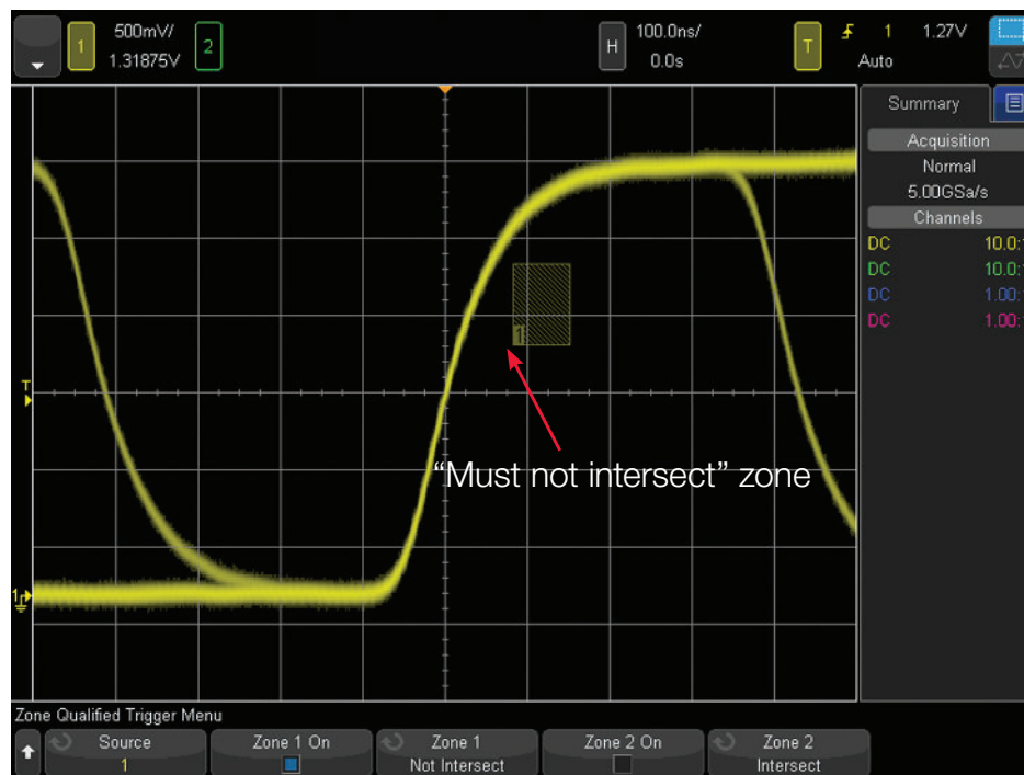
Figure 3. Capturing and displaying just waveforms with “normal” edges using Zone Trigger.
