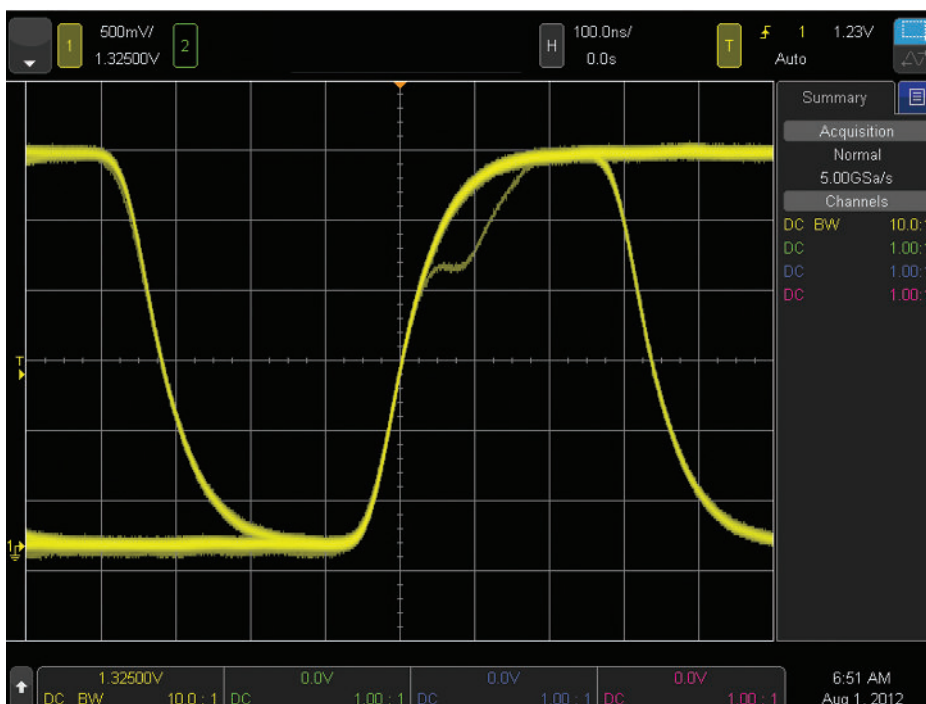
Figure 1. Capturing a signal with an infrequent non-monotonic edge using standard edge triggering.
