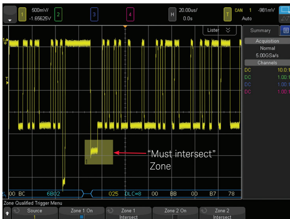
Figure 11. Using Zone Trigger to synchronize on just frames that include arbitration.
