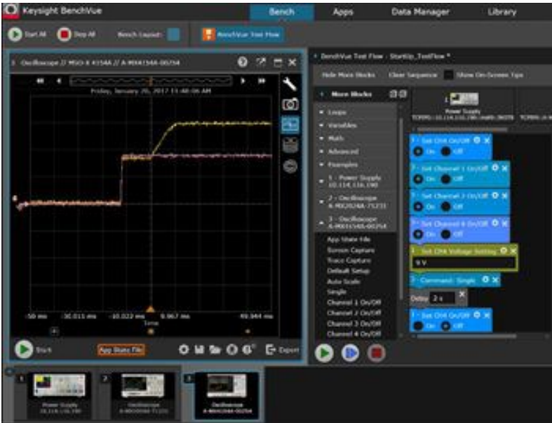
Figure 7. BenchVue start-up test flow, B) Results of a start-up test, time-based measurement
