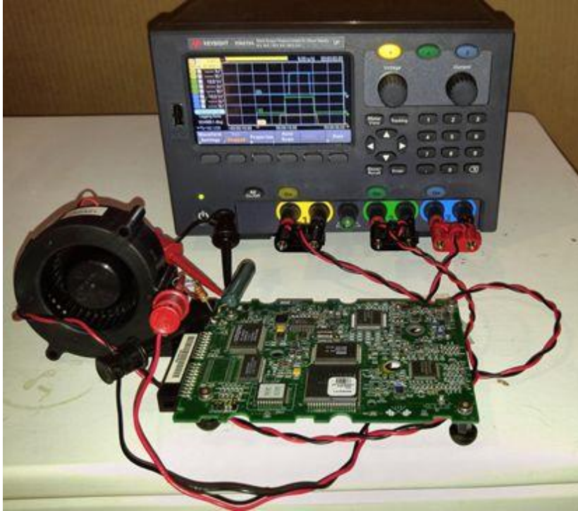
Figure 1. The E36313A triple-output bench power supply connects to power up a circuit board
