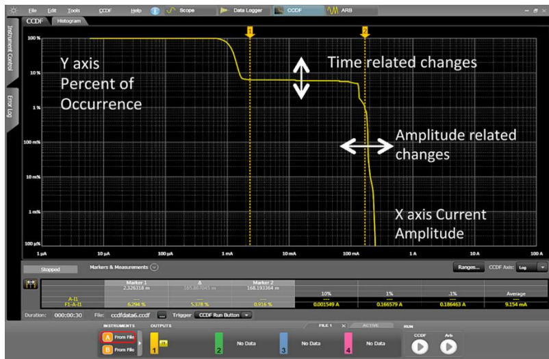
Figure 8. CCDF measurement reveals the key attributes of standby current in a smartphone
