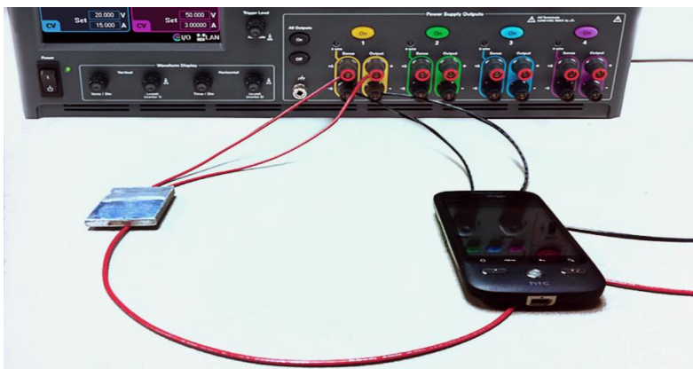
Figure 2. The setup for measuring battery drain performance using the N6781A or N6785A SMU installed as output 1 in an N6705 DC power analyzer
