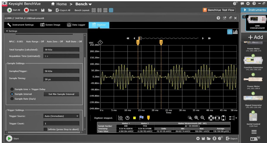
Figure 7. PathWave BenchVue's digitizing function screen
