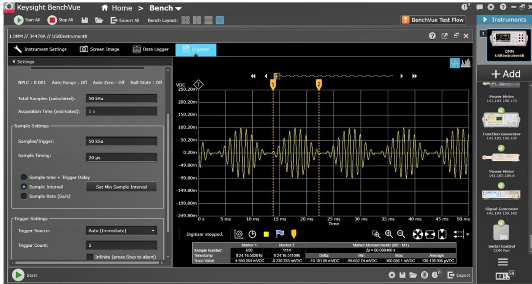
Figure 7. PathWave BenchVue's digitizing function screen
