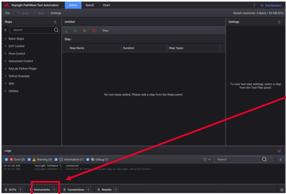
To add an instrument to a test automation in the Digital Learning Suite software, click the '+' add sign at the bottom of the Test Automation homepage and select the type of instrument.
