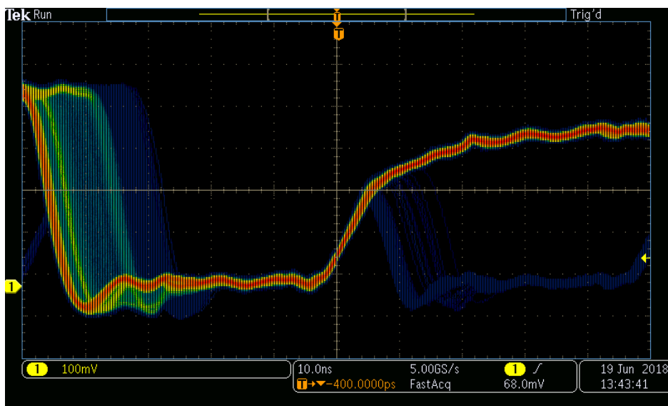
Figure 5. Tektronix MDO3000 Series scope captures the event with FastAcq acquisition mode on while updating at a rate of 280,000 waveforms/s.
