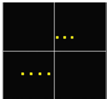
Figure 27. Waveform where the sample rate yields two data points per period.
