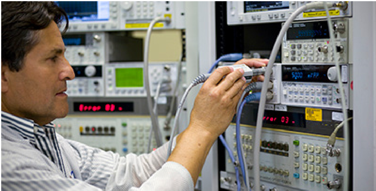
Figure 1. Test engineer installing DMM in a manufacturing test system
