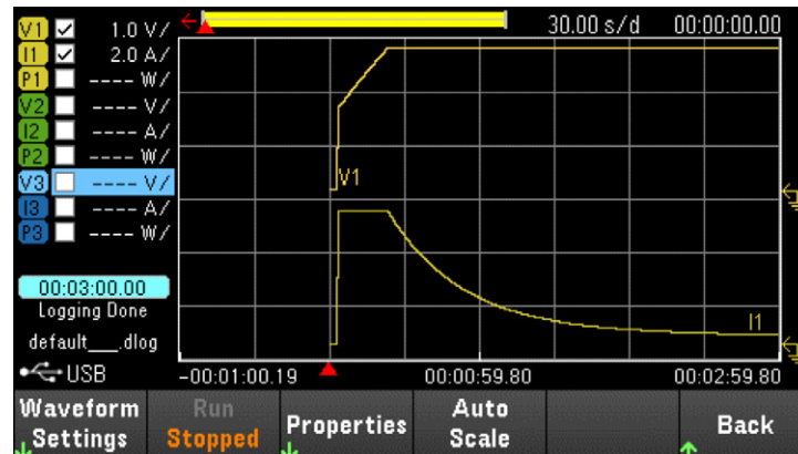
Figure 2. The E36312A capturing the charging of a 100 F supercapacitor
