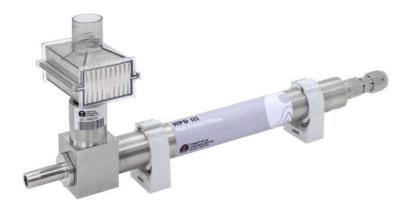
High Pressure Diffusers (HPDs) have been developed to address the challenge of sampling pressures of  $5-100~\rm psi$ , and the possible damage that can result from connecting pressurized air or gas to a particle counter. HPDs reduce the pressure of the gas to near atmospheric pressure by allowing some of the gas to diffuse out of the system, allowing the particle counter's flow-metering system to function as designed.
