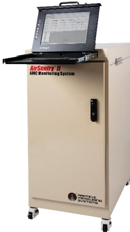
The AirSentry® II Multi-point Monitoring System is the most advanced airborne molecular contamination (AMC) monitor available, utilizing sensitive and responsive ion mobility spectrometry to detect and characterize airborne molecular contamination from multiple locations within a cleanroom. The system features a 16- or 30-point manifold sampling system and an on-board industrial computer with secure software and communications.
