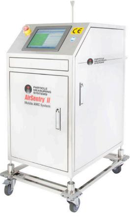
Designed to enhance fixed AMC monitoring programs, the AirSentry II Mobile AMC Detection System is the first truly mobile system for monitoring airborne molecular contamination in cleanrooms. Mobility plays an important part in a strategic AMC monitoring program, allowing contamination sources to be quickly located, quantified and eliminated.
