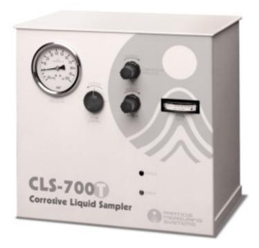
The CLS-700 T corrosive liquid sampler is a compression sampler combined with a LiQuilaz® particle counter for effective measurement of particles in fluids contained in unpressurized vessels. It is ideally suited for testing effervescent chemicals. The system eliminates bubbles by pressurizing the sample and forcing the bubbles into solution.
