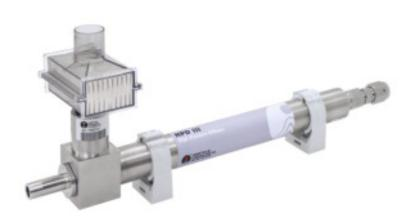
High Pressure Diffusers (HPDs) have been developed to address the challenge of sampling pressures of 5 – 100 psi, and the possible damage that can result from connecting pressurized air or gas to a particle counter. HPDs reduce the pressure of the gas to near atmospheric pressure by allowing some of the gas to diffuse out of the system, allowing the particle counter's flow-metering system to function as designed.
